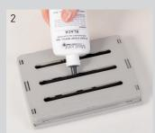
Select right colour of MaxLight re-fill ink and add a few of drops into slotted back of die box.
